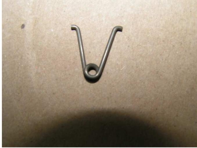
**The only critical issue while installing the spring is to be certain that the “LONG” leg of the spring MUST be placed into the detent in the FRAME of the block, then obviously, the short leg attaches into the lever drum detent. Yes, one IS longer! Notice it is on the right side in the above picture. It isn’t that much longer, but it is longer and it has to be against the frame for it to work properly.**
