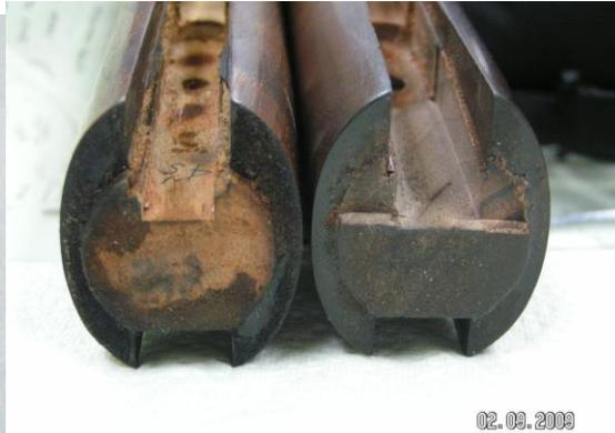
Remove the tang through screw and insert the unit into the stock. Use a scribe or sharp pencil to mark the area to be removed (see fig. #4) then, remove the excess wood all the way to the existing relief line. You can use whatever tools you have to trim the nose flat with the shoulder of the Butt Stock (see fig #5). A simple wood rasp will do it in about two minutes, a small fine toothed saw will take about the same time. Be careful! Some inletting may be necessary later to get the stock to fit.
